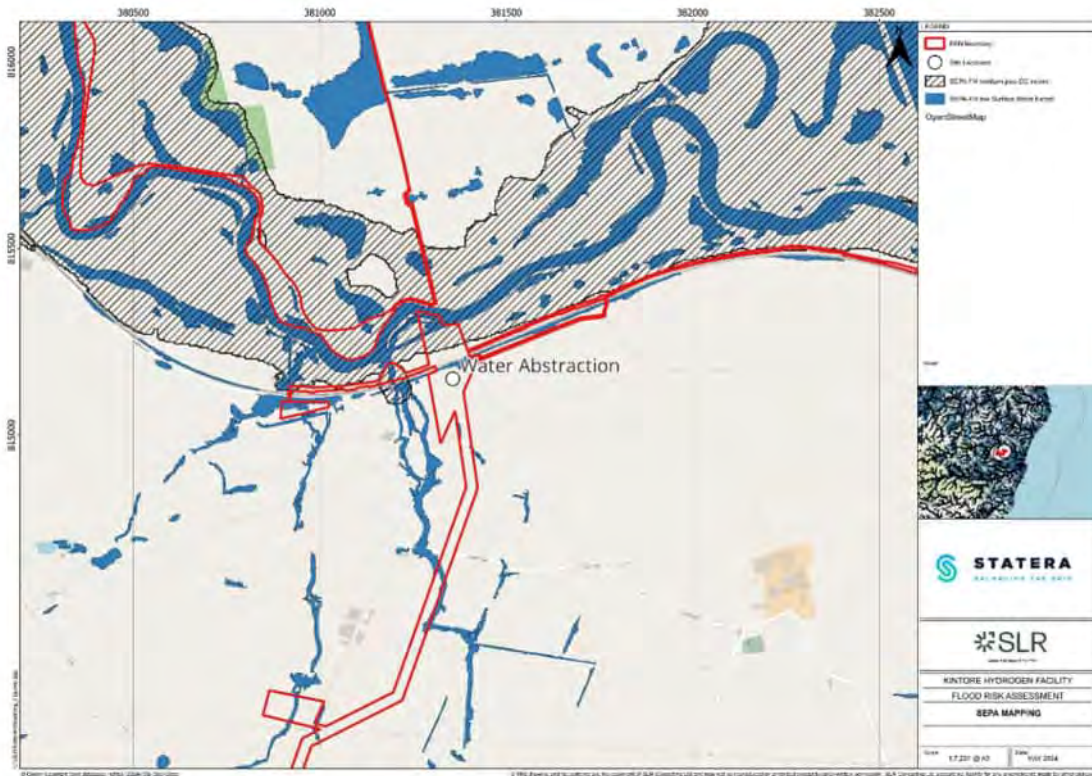
Figure 2-3 – SEPA River and Surface Water Flood Mapping at the water abstraction and treatment plant
