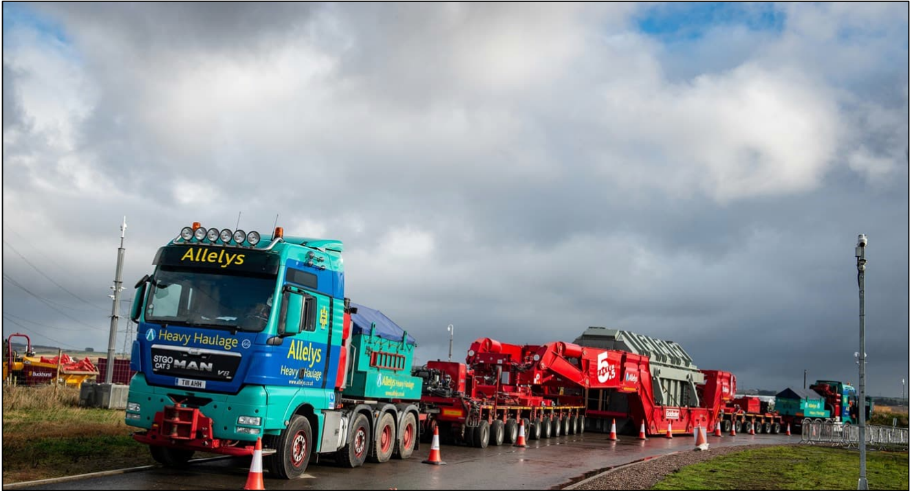
Figure 2-2: Example Transformer Transport
