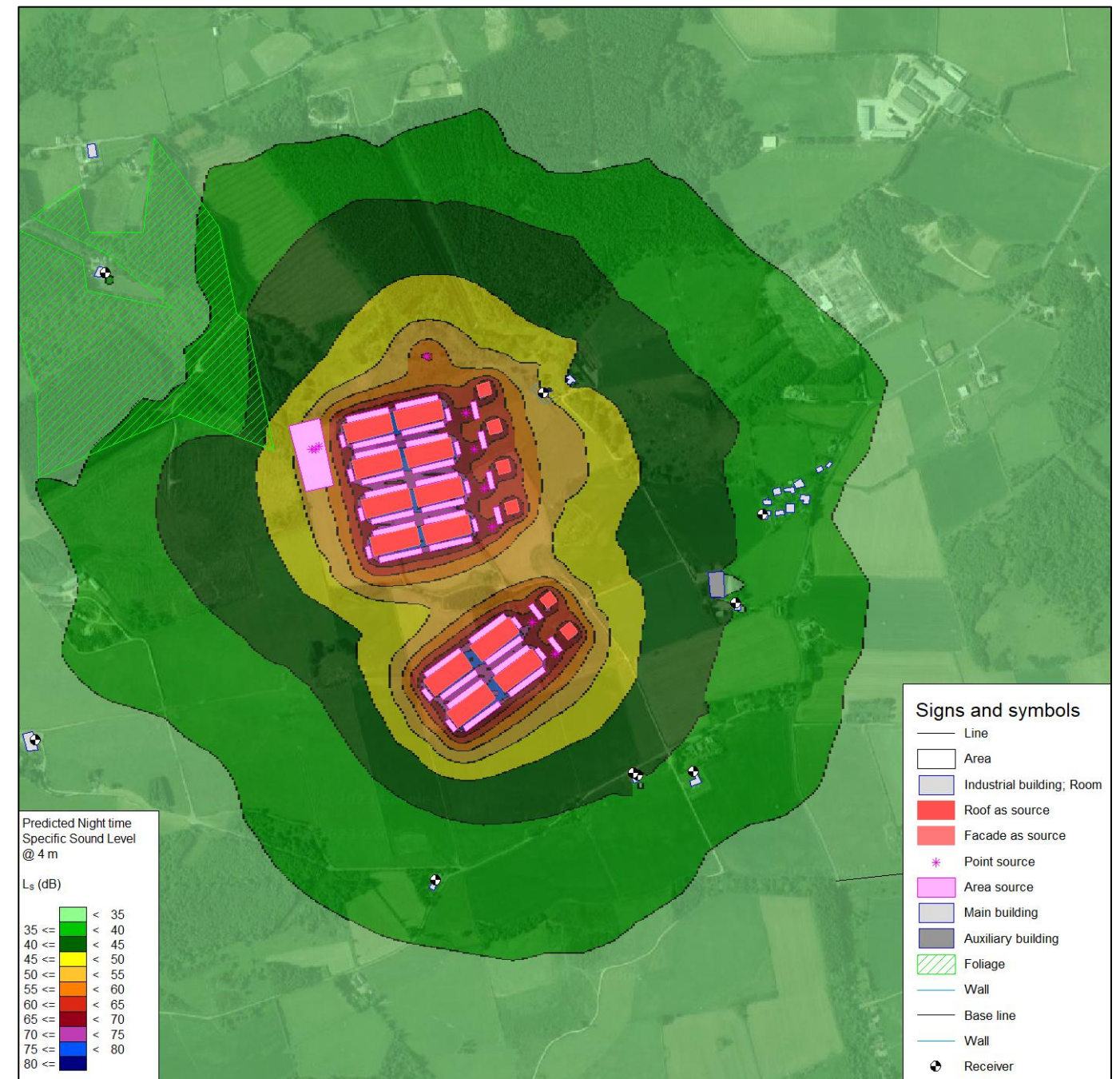
Figure 4.1: Operational night-time noise contour from electrolysis plant
